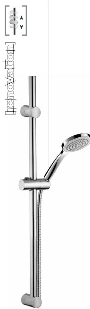
Slide rail in brass, Ø .7", with swivel bracket in abs, flexible metal shower hose, 59" length, connection 1/2", handshower in abs. max flow: 1.8 GPM.
