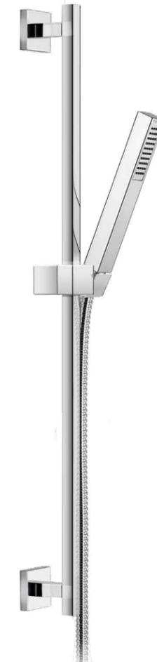
· Slide rail in brass, Ø .7", with swivel bracket in abs, flexible metal shower hose, 59" length, connection 1/2", handshower in abs. max flow: 1.8 GPM.
