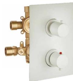
• **Rough In,** 3/4" concealed thermostatic valve for shower with built-in 3/4" ceramic discs diverter, 3 outlets, stop function and volume control. flow rate: 10 GPM (45 PSI).
