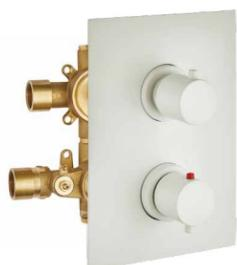
• **Rough In,** 3/4" concealed thermostatic valve for shower with built-in 3/4" ceramic discs diverter, 2 outlets, stop function and volume control. flow rate: 10 GPM (45 PSI).
