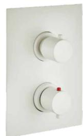
• **Complete** 3/4" concealed thermostatic valve for shower with ceramic discs diverter, 3 outlets, stop function and with volume control. flow rate: 10 GPM (45 PSI).
