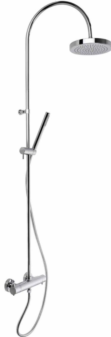
· Slide rail in brass, .6" x .6", with swivel bracket in abs, flexible metal shower hose, 59" length, connection 1/2", handshower in abs. max flow: 1.8 GPM.
