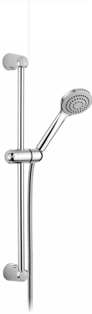
Slide rail in brass, Ø .7", with swivel bracket in abs, flexible metal shower hose, 59" length, connection 1/2", handshower 3 jets spray in abs. max flow: 1.8 GPM.
