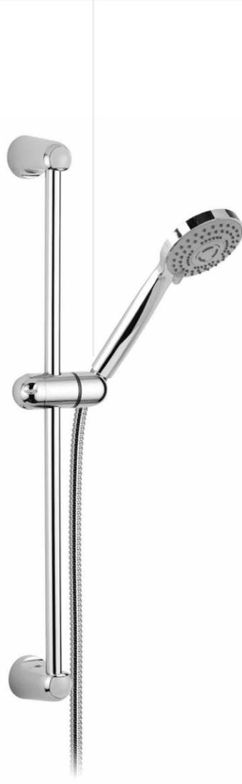
Slide rail in brass, Ø .7", with swivel bracket in abs, flexible metal shower hose, 59" length, connection 1/2", handshower in abs. max flow: 1.8 GPM.
