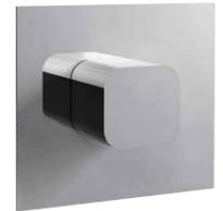
• **Complete** concealed stop valve 3/4" ceramic discs 90° with volume control. flow rate: 13 GPM (45 PSI).
