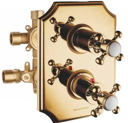
• **Rough In**, 3/4" concealed thermostatic valve for shower with built-in 3/4" ceramic discs diverter, 3 outlets, stop function and volume control. flow rate: 10 GPM (45 PSI).
